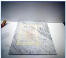
2) Apply PLATINUM STAIN OUT using a brush directly on the oxidation / humidity stain.
